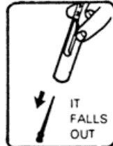
10 Remove firing pin through rear of bolt carrier
